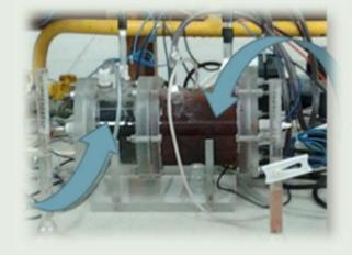
A dual-chamber (H type), two electrode fuel cell was used to monitor the biocatalyzed generation of electricity.
